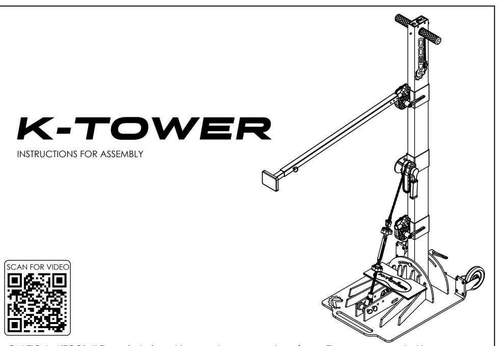
CAUTION – KECO's K-Tower is designed to operate on concrete surfaces. The vacuum created by the air supply may cause damage to floors comprised of layers or different substrates. This would include, but not limited to, decorative flooring, tile, and athletic-sport surfaces.
